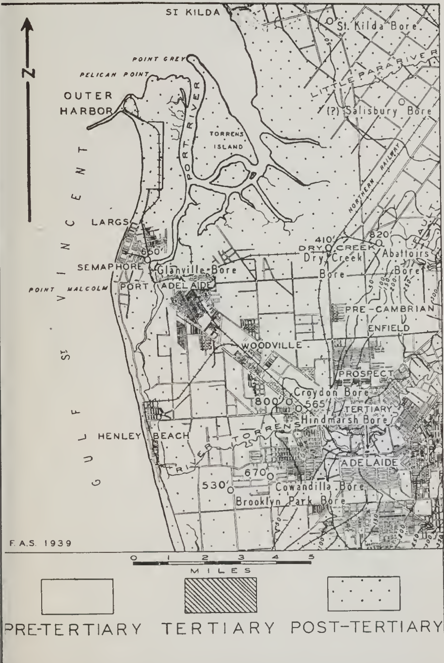
FIG. 2.—Geological map of Adelaide district, South Australia, with sites of bores cutting Adelaidean beds. Contours from Adelaide sheet, Military Survey of Australia, 1915.
